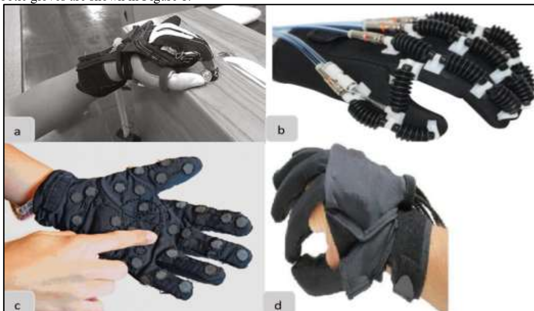
Figure 1: Different types of soft gloves: (a) soft robotic glove [10], (b) pneumatic soft robotic glove [11], (c) smart tactile glove [12], (d) pneumatic robotic glove [13]
