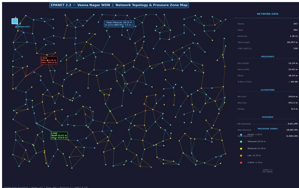
Figure 2: EPANET 2.0 — Network Topology Map of Veena Nagar WDN (357 Nodes, 492 Pipes) Red dots = Critical pressure nodes (<15 m); Orange = Marginal zone nodes; Blue = Reservoir R-1
