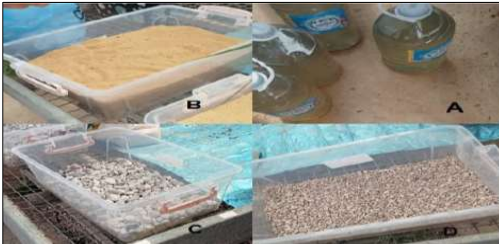
Fig. 3 Composition of the experimental setup. A: wastewater samples; B: sand layer sand; C: layer of coarse gravel; D: layer of fine gravel
