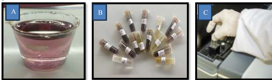
Figure 2: Anti-oxidant assay, A) DPPH solution, B) Sample preparation, C) UV analysis
