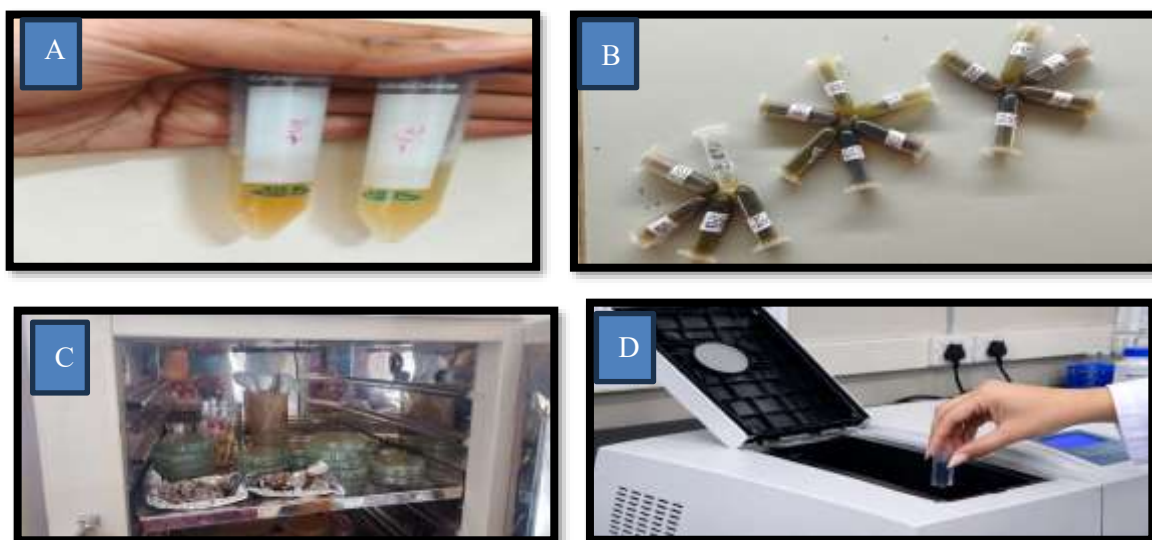
Figure 1: Antimicrobial test ,A) Bacterial solution,B) Preparation of Samples,C) Kept in Incubator,D) UV Analysis
