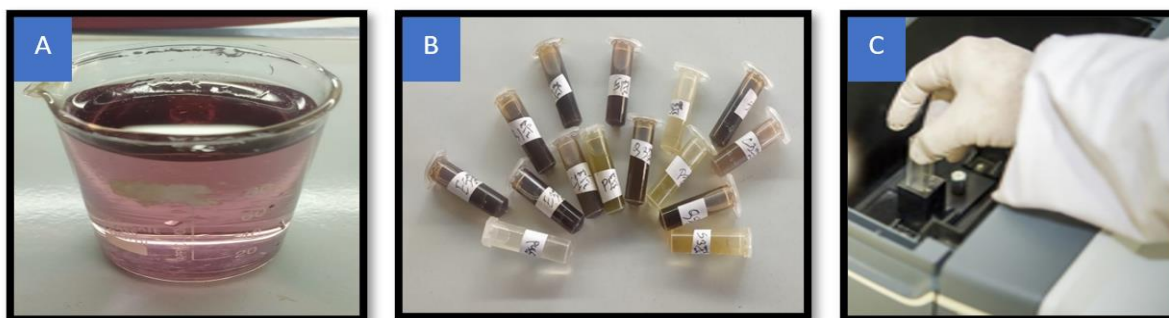
Figure 2: Anti-oxidant assay, A) DPPH solution, B) Sample preparation, C) UV analysis
