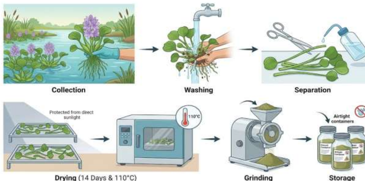
Figure 2. Schematic workflow of the step-by-step sample preparation procedure for water hyacinth ( Eichhornia crassipes )
