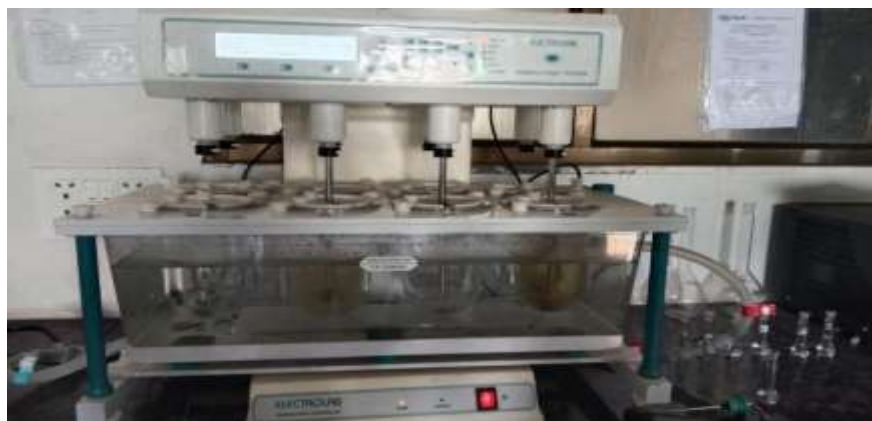
Fig :- Dissolution Tester
