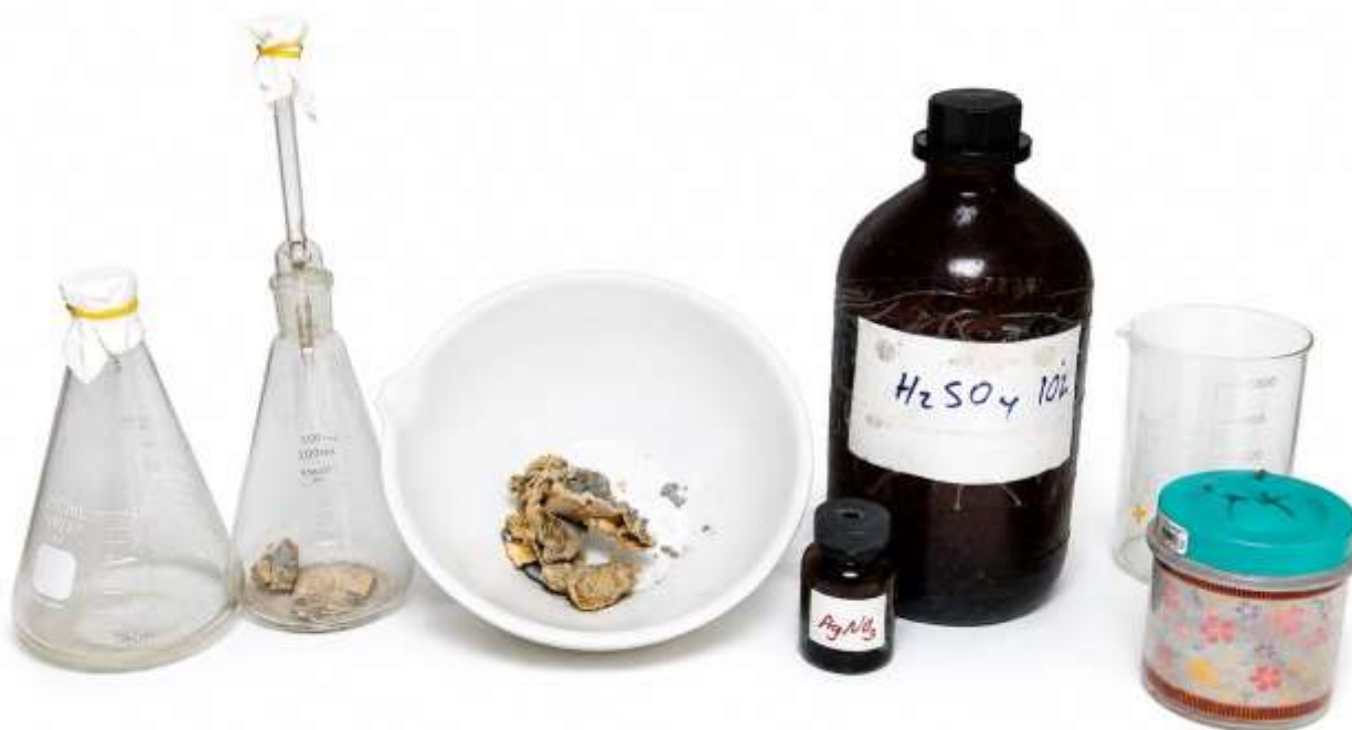
Figure 1: Laboratory technique for the Silver Nitrate Spot Test
