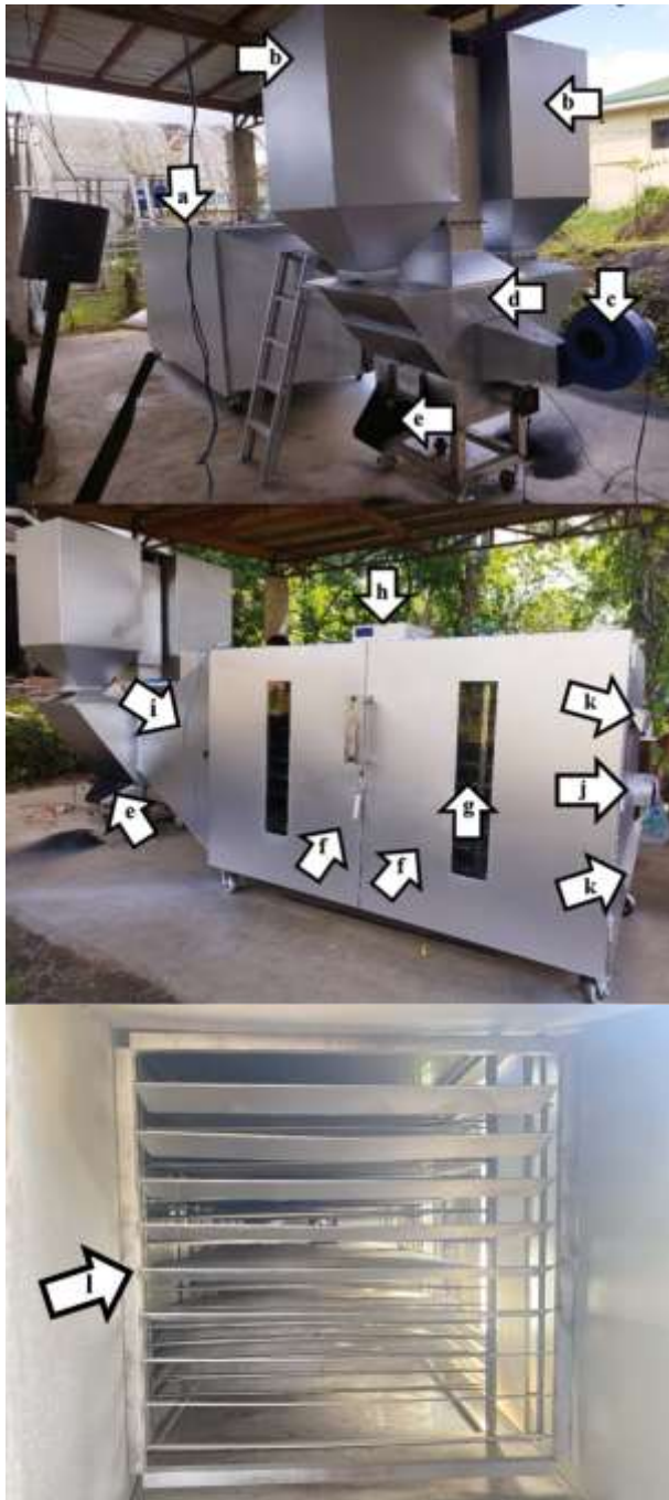
Fig. 2. Different parts of the multi-layer biomass-fired fish dryer include the following: (a) drying cabinet, (b) biomass holding bins, (c) blower, and (d) biomass furnace, (e) ash outlet, (f) cabinet doors, (g) drying trays, (h) control and indicator, (i) expanding air duct, (j) backdraft damper, (k) exhaust vents, and (l) baffle assembly.
