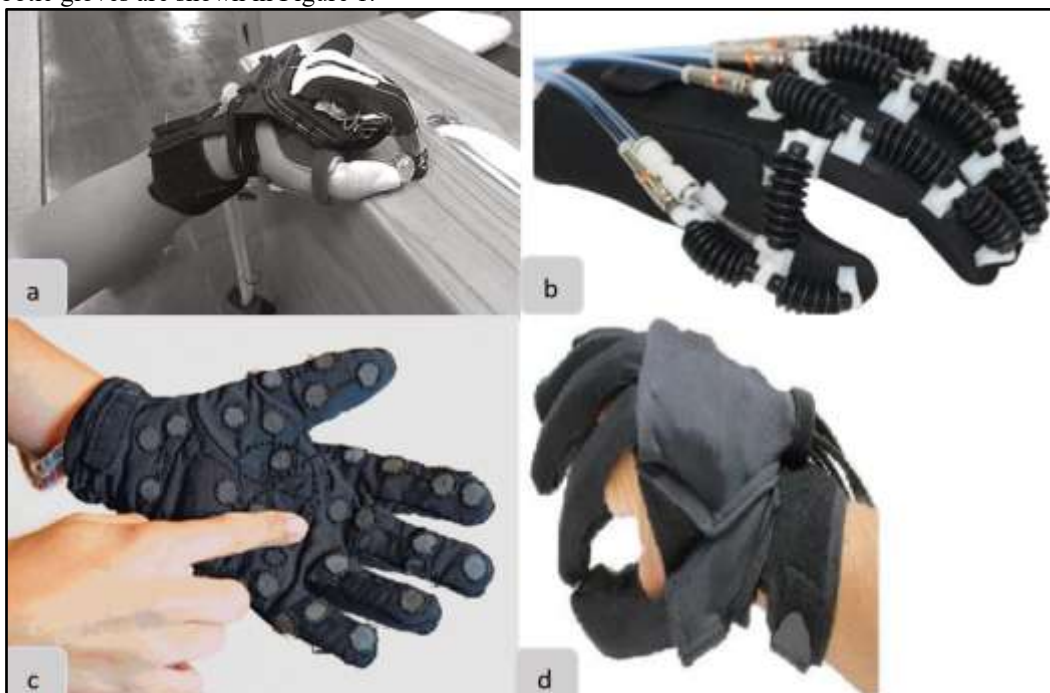
Figure 1: Different types of soft gloves: (a) soft robotic glove [10], (b) pneumatic soft robotic glove [11], (c) smart tactile glove [12], (d) pneumatic robotic glove [13]
