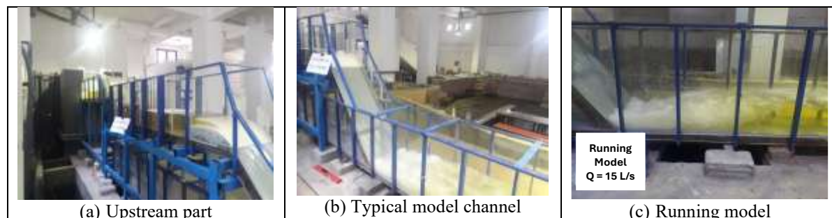
Figure 1. The layout of the hydraulic model in the laboratory
